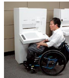
Testing a public information terminal. Many different types of people were enlisted to test the terminal from early in the development stage. The views of experts were also incorporated into the design.
