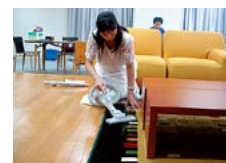
Testing of a vacuum cleaner by the visually impaired. Workshops are conducted in which people use products in order to test usability and find unnoticed problems.
