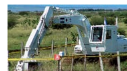
The anti-personnel mine remover in use in Nicaragua. After mine removal, the land will be used for orchards, etc.
