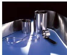
Amorphous alloys for transformers by Hitachi Metals, Ltd.
