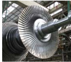
Ultra supercritical steam turbine
