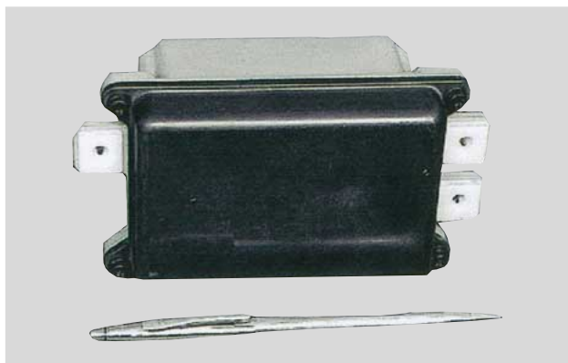
Fig. 6—Appearance of the Developed Millimeter-Wave Radar. The radar unit is more compact than the conventional product and is easily mounted on an automobile.
