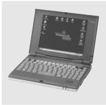
Fig. 5— Handheld HPW-600JC PC. VGA (video graphics array) screen and keyboard-type handheld PC equipped with an SH7500 SuperH RISC engine. First introduced in 1999 along with tablet-type PCs.
