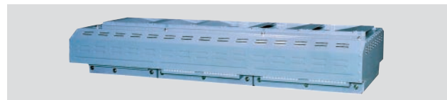
Fig. 4—External Appearance of Battery Box. Fitted on the roof of the train carriages, the battery box is fitted with heat-shield panels to stop heating of the equipment inside it by direct sunlight.
