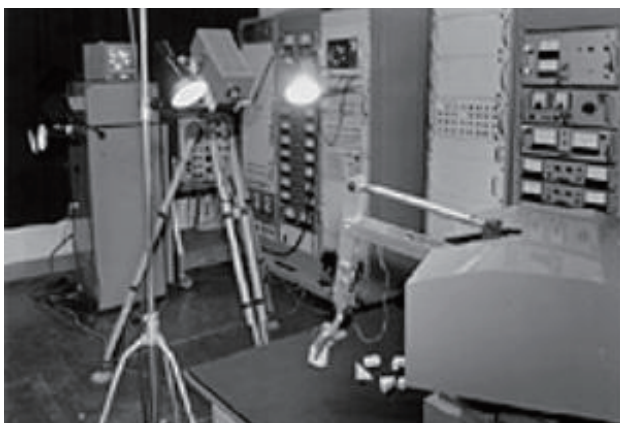
Fig. 2—HIVIP Mk.1 Prototype Intelligent Robot. Hitachi developed the first integrated intelligent robot in 1970. The robot captures video images of engineering drawings, understands the purpose of the tasks given to it, recognizes objects (building blocks) on the table, plans the sequence of motions to execute the task, and then automatically assembles the objects as shown in the drawings.
